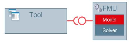
The FMI defines an interface to be implemented by an executable called Functional Mock-up Unit (FMU)
